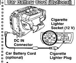
Connect PV-C16 <u>Car Battery Cord</u> (optional) to <u>Camcorder DC IN</u>.
