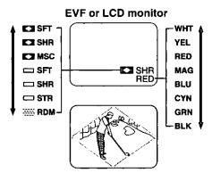
■ For more effects, stop fade in or fade out at any time (except RANDOM mode) by pressing <u>FADE</u>. Then, press <u>FADE</u> to resume fade.
