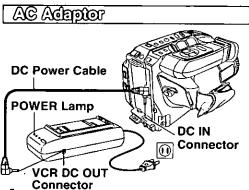
Connect AC Adaptor VCR DC OUT to Camcorder DC IN with supplied DC Power Cable.
