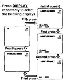
Tape remaining indicator operates a few seconds after tape starts moving.
